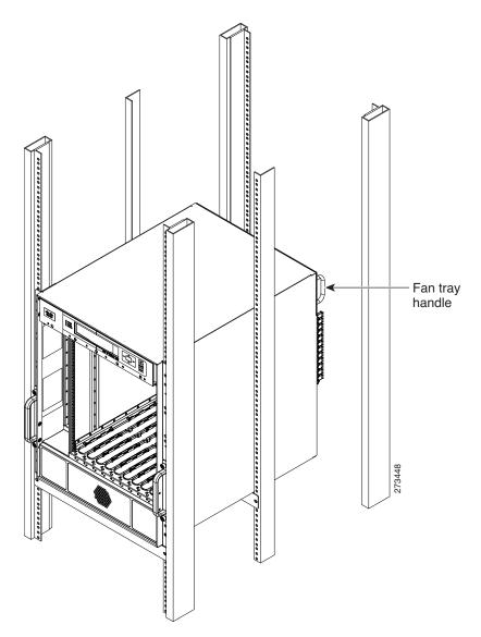
**Step 7** Hold the chassis in position against the mounting rails and follow these steps:
